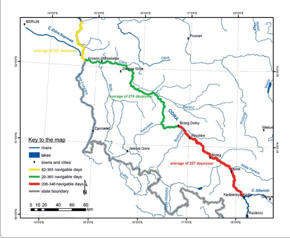
However, it should be noted that the above-described results do not take into account the limitations of navigation related to icing, too-small radiuses of meanders and the occurrence of too-high water levels, when navigation is impossible because of inadequate clearances beneath bridges.
