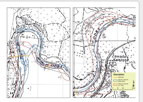
The reach between the confluence of Lusatian Neisse and the confluence of Warta has the best rate of accomplishment of parameters for a waterway of Class III. The most significant reconstruction works would be necessary between Brzeg Dolny and the confluence of Lusatian Neisse.
