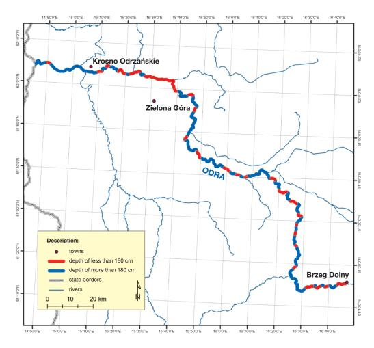
Minimum transit depth of a waterway of Class III at the stretch of the Odra from Brzeg Dolny to the confluence of Lusatian Neisse in an average year. Fragments of the riverbed, where the minimum transit depth achieves 1.8 m for at least 240 days (as required for a waterway of Class III) in an average year have been marked in blue. Other reaches of the Odra do not meet the parameters of Class III.
