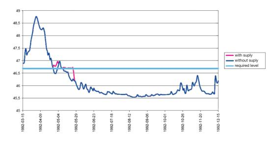
It was estimated that the compensation of very low water in 1992, 2003, and 2004 would require a capacity of about 2000 million m<sup>3</sup>, 2400 million m<sup>3</sup> and 2200 million m<sup>3</sup> respectively. A significant extension of the navigation period would therefore, require immense additional capacity of reservoirs, impossible to attain considering spatial, financial, and environmental issues.
